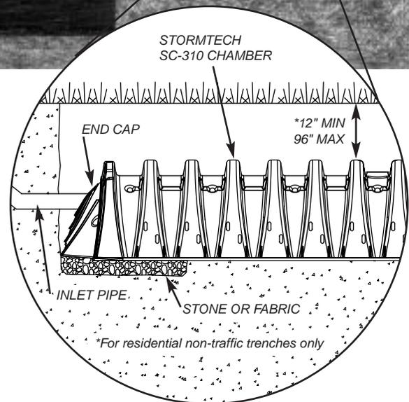
**Safety.** Because the chambers are underground, they eliminate erosion ditches and potential hazards caused by conventional roof drains and ice build-up in the winter.
